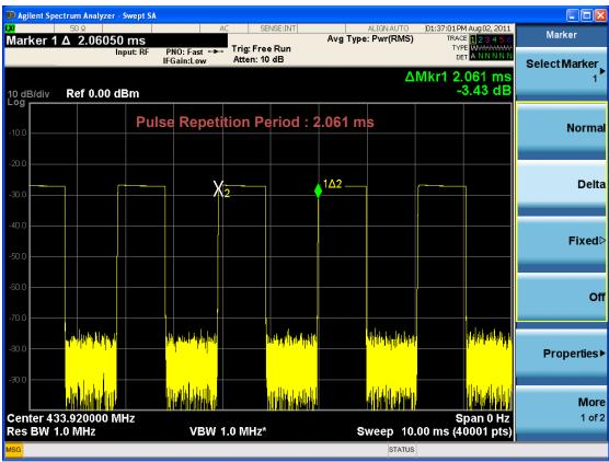
Average Factor 2 =  $20 \log \left[ \frac{0.978 \text{ ms}}{2.061 \text{ ms}} \right] dB = -6.47 \text{ dB}$
