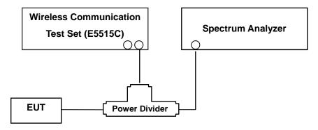
(Configuration of conducted Emission measurement) Test Procedure
