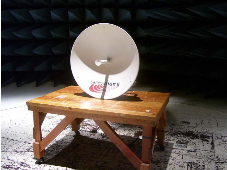
Photograph 3. Test Equipment and setup for various Radiated Measurements Parabolic Antenna
