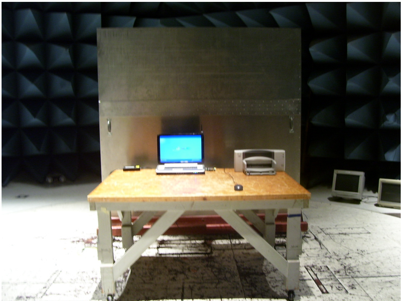
Photograph 2. Conducted Emissions Test Setup – Front View
