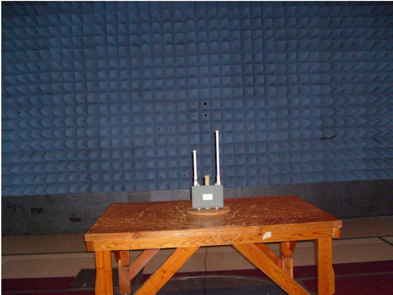
Photograph 1. Spurious Radiated Emissions, Test Setup
