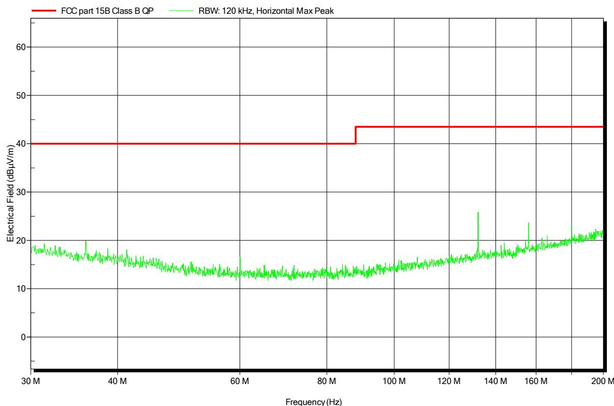
**Spurious emissions under normal conditions according to FCC 15B**
