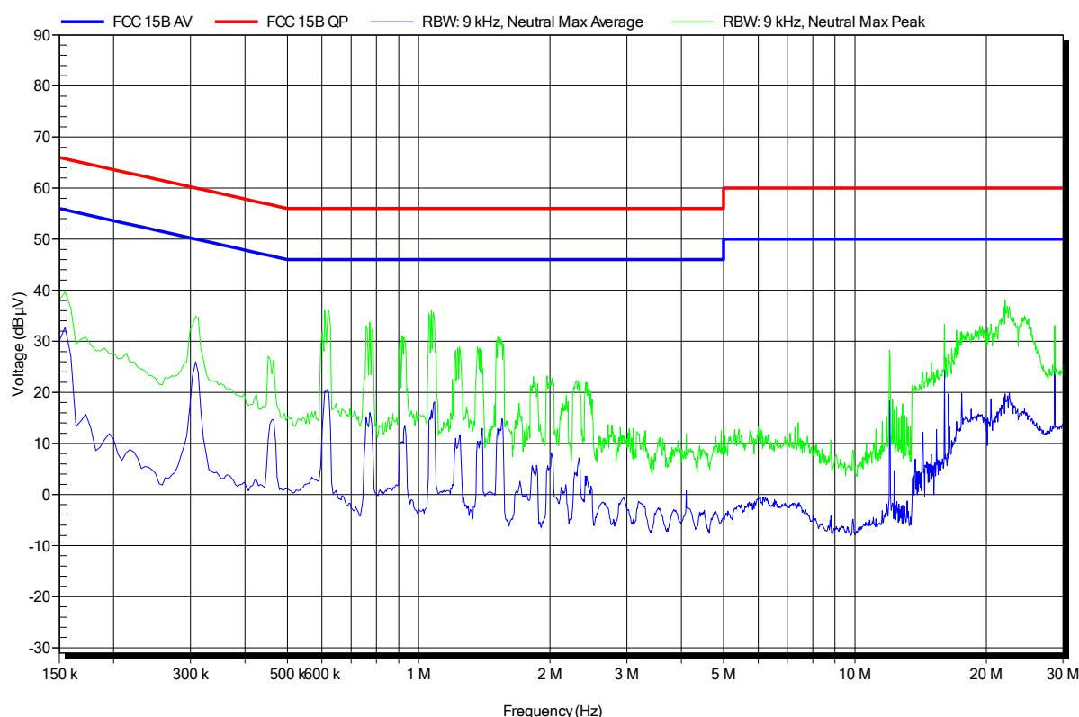
**EMI voltage test in the ac-mains according to FCC 15B**
