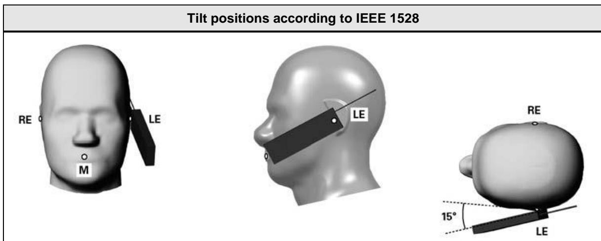
First the EUT is placed in the cheek position. Next the handset is moved away from the pinna along the line passing through RE and LE far enough to allow a rotation of the handset away from the cheek by 15°. Then the handset is rotated around the horizontal line by 15°.
