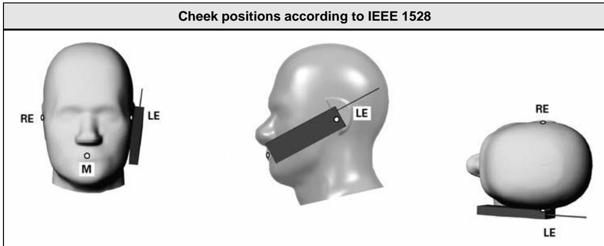
The handset is positioned close to the surface of the phantom such that point A is on the (virtual) extension of the line passing through points RE and LE on the phantom (see Figure), such that the plane defined by the vertical centerline and the horizontal line of the handset is approximately parallel to the sagittal plane of the phantom. Next the handset is translated towards the phantom along the line passing through RE and LE until handset point A touches the pinna at the ERP.
