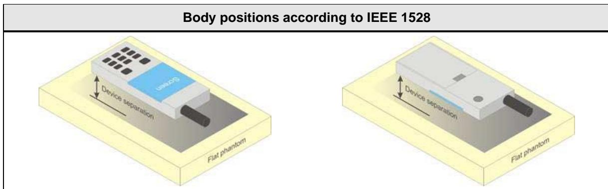
In body worn configuration the device is positioned parallel to the phantom surface with either top or bottom side of the EUT facing against the phantom.
