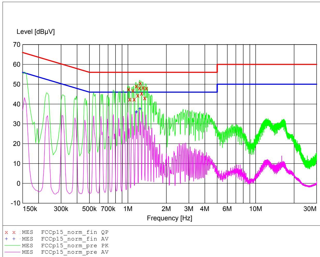
**EMI voltage test in the ac-mains according to FCC part 15**
