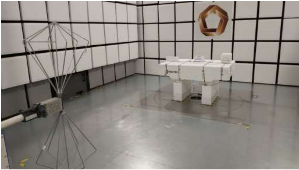
TEST SETUP PHOTO(S) - RADIATED MEASUREMENT / 30MHZ TO 200MHZ
