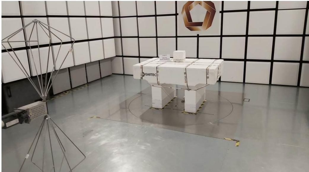
TEST SETUP PHOTO(S) - RADIATED MEASUREMENT / 30MHz TO 200MHz
