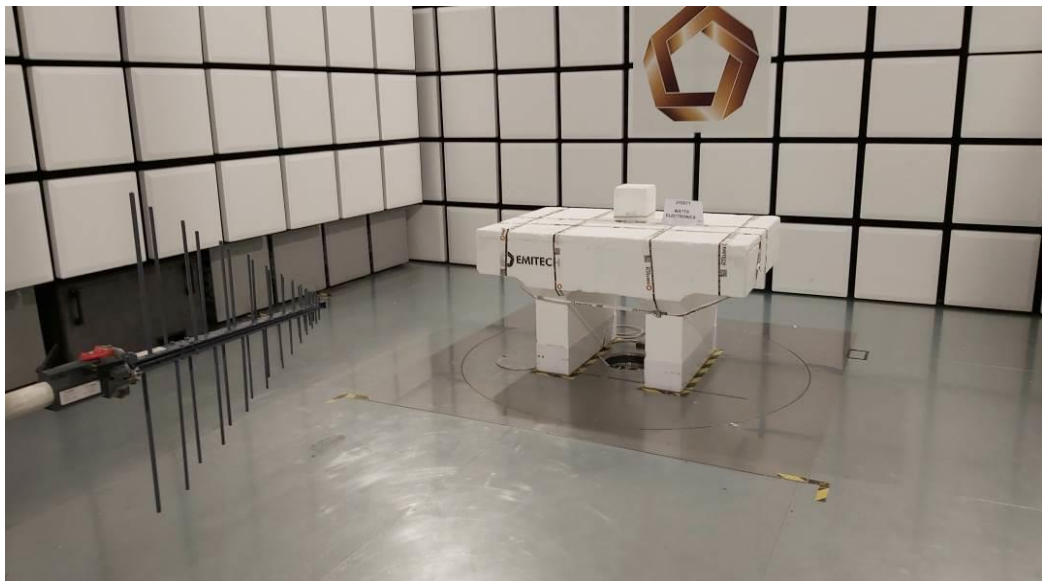
TEST SETUP PHOTO(S) - RADIATED MEASUREMENT / 200MHz TO 1GHz
