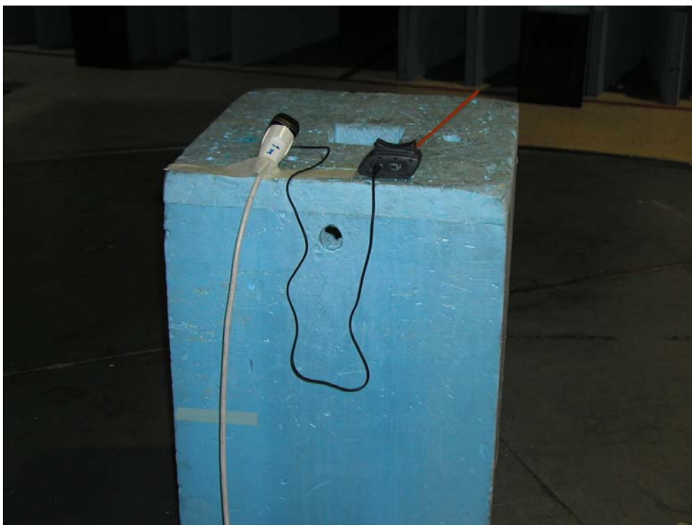
Photograph 4. Spurious radiated emissions-unintentional radiator test setup
