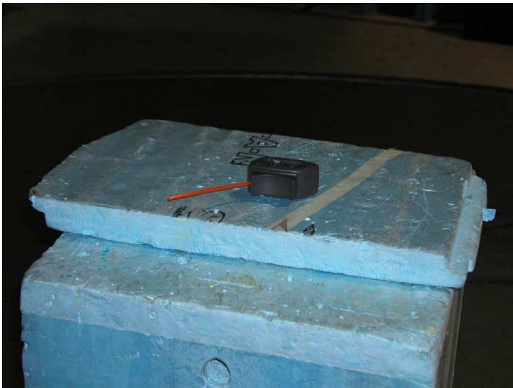
Photograph 2. Radiated RF output power and spurious radiated emissions test setup
