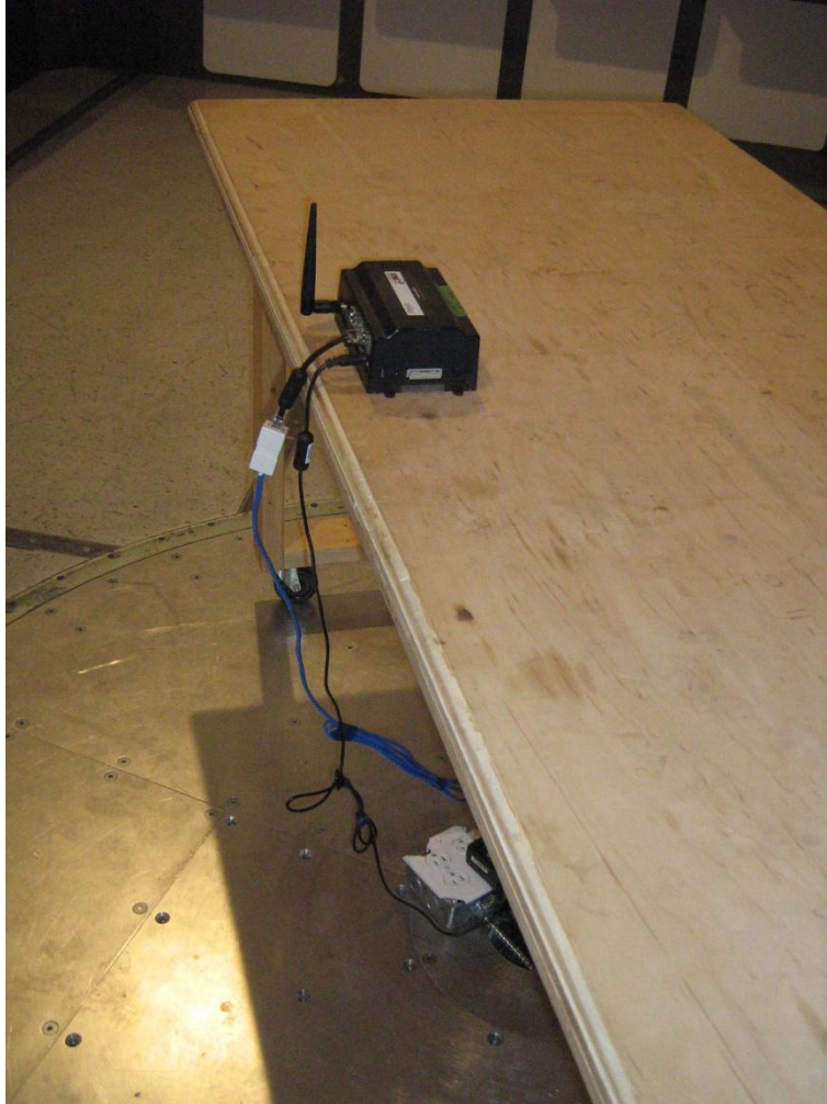
Figure 2 – Radiated emission setup
