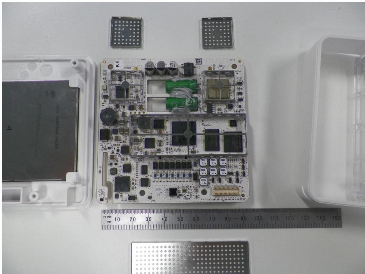
PCB Primary Side No Shield covers + shield supports cut off
