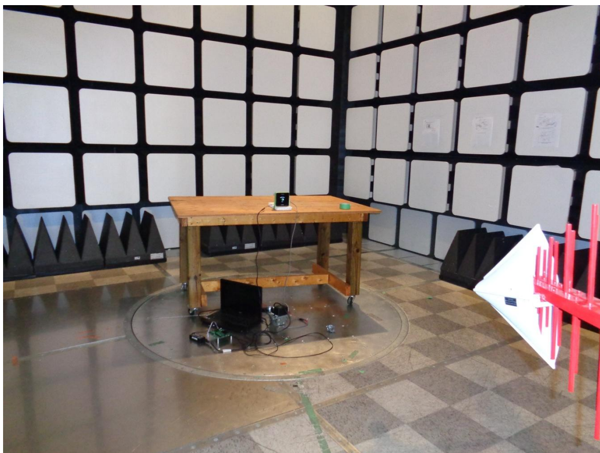
Radiated Emission Test Setup Photo #1:
