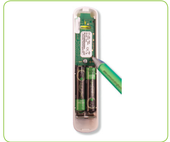
Figure-5 Shorting the Switch
