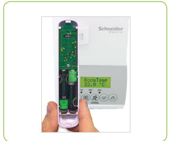
Figure-6 Switch/Controller Proximity During Pairing
