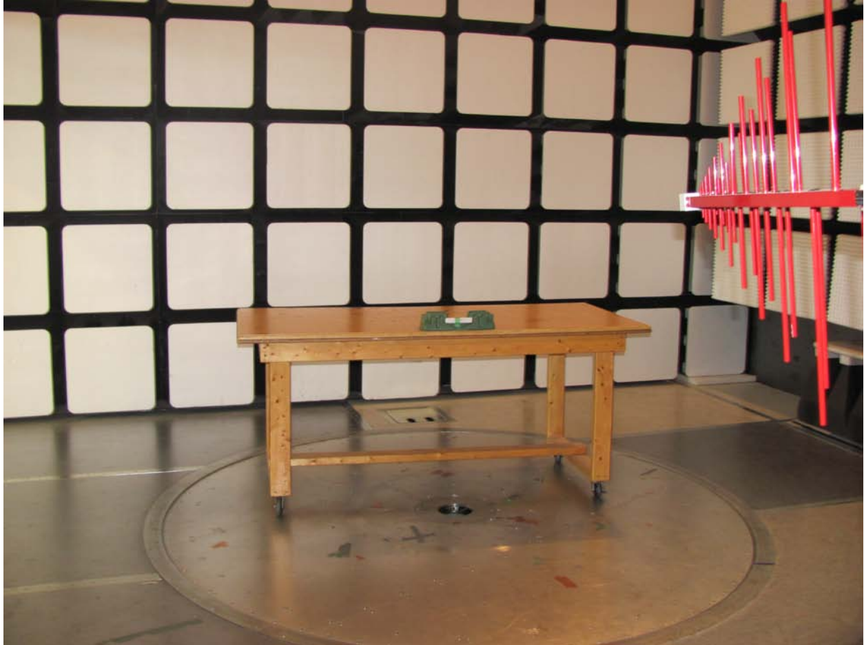
Illustration 2: Radiated emission setup - photo 2
