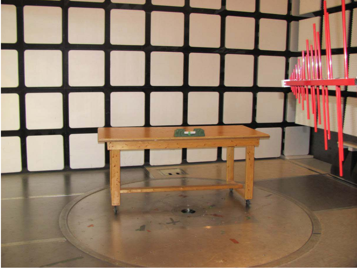
Illustration 7: Radiated emission setup - photo 2
