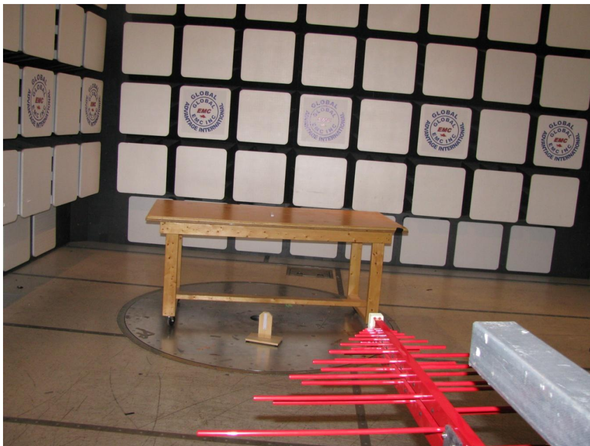
Figure 1 – Radiated emission setup
