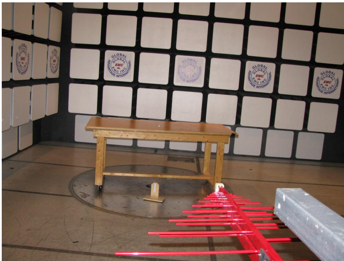
Figure 1 – Radiated emission setup
