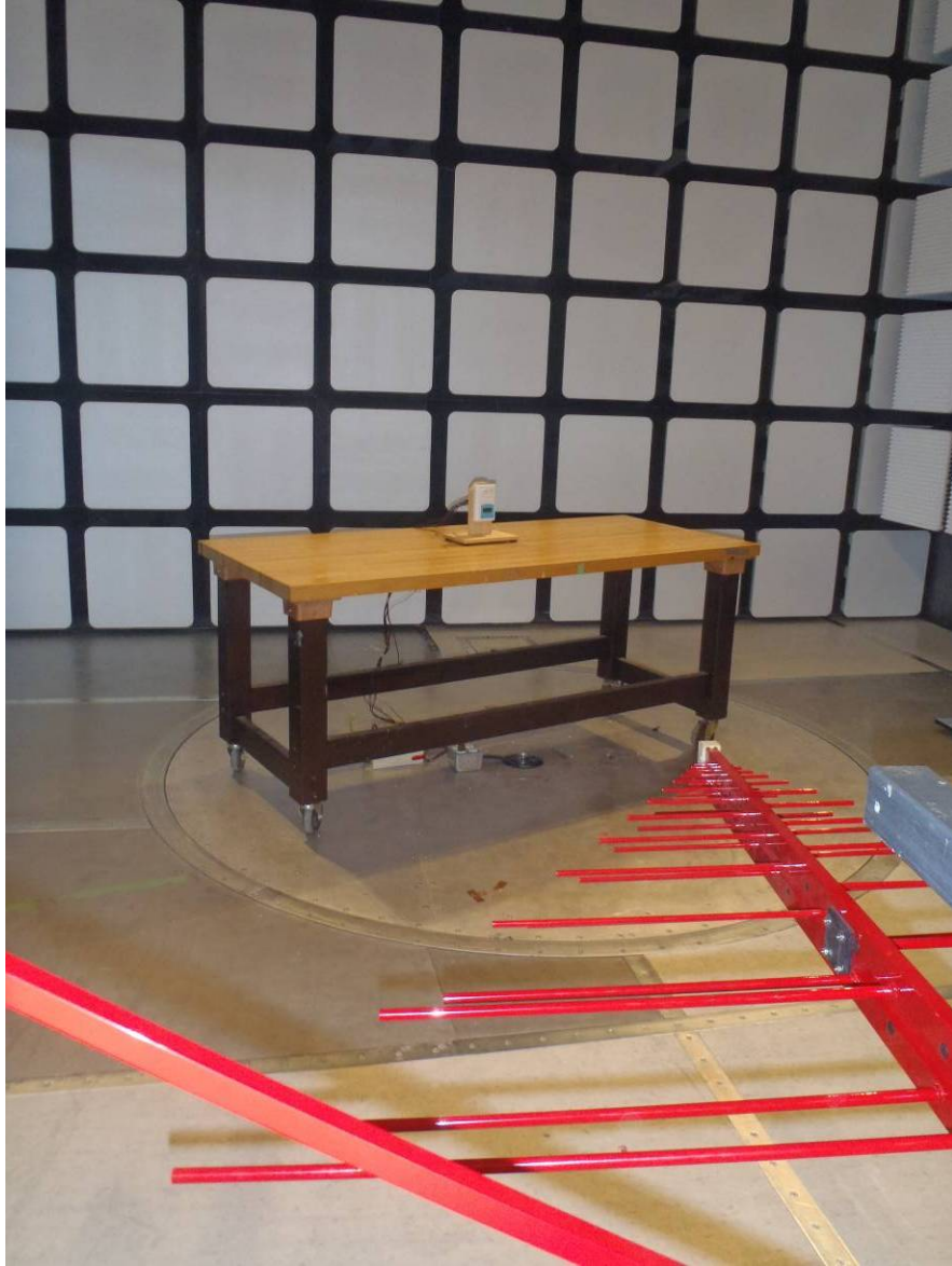
Radiated Emissions – 30 MHz to 1 GHz
