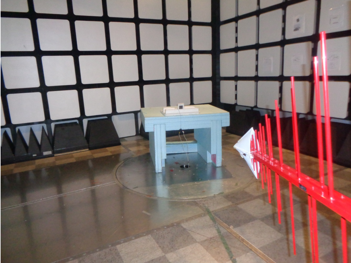
Figure 1 – Radiated Emissions Setup – Photo 1
