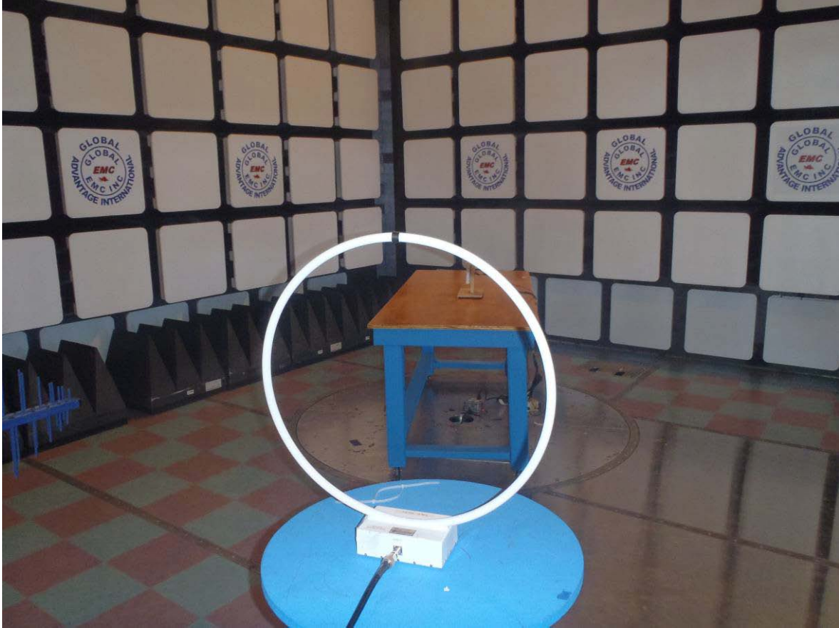
Illustration 3: Radiated emission setup – photo 1
