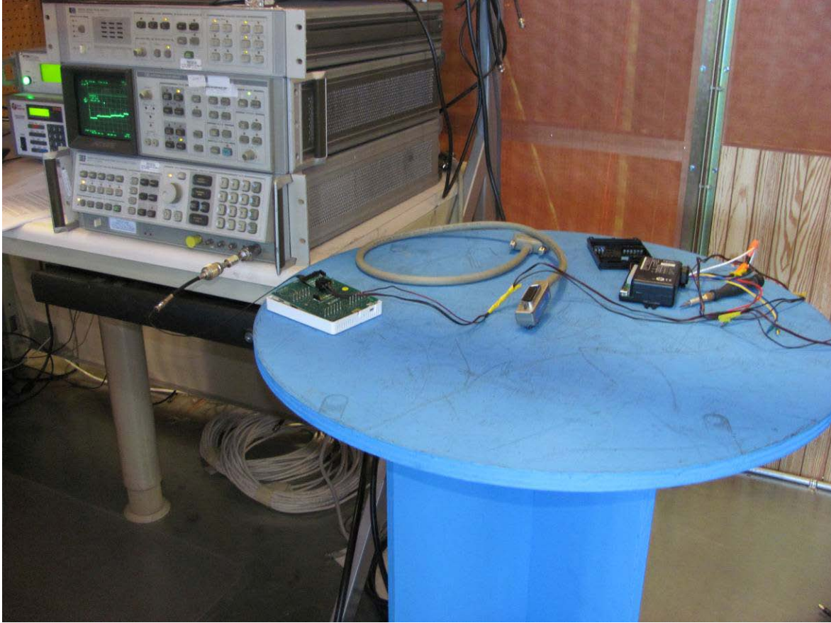
Illustration 6: Antenna conducted emission setup
