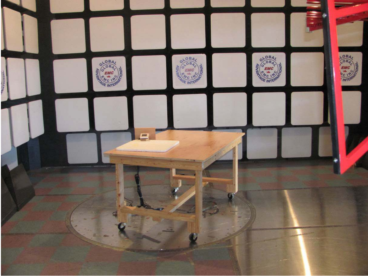
Illustration 4: Radiated emission setup - photo 2
