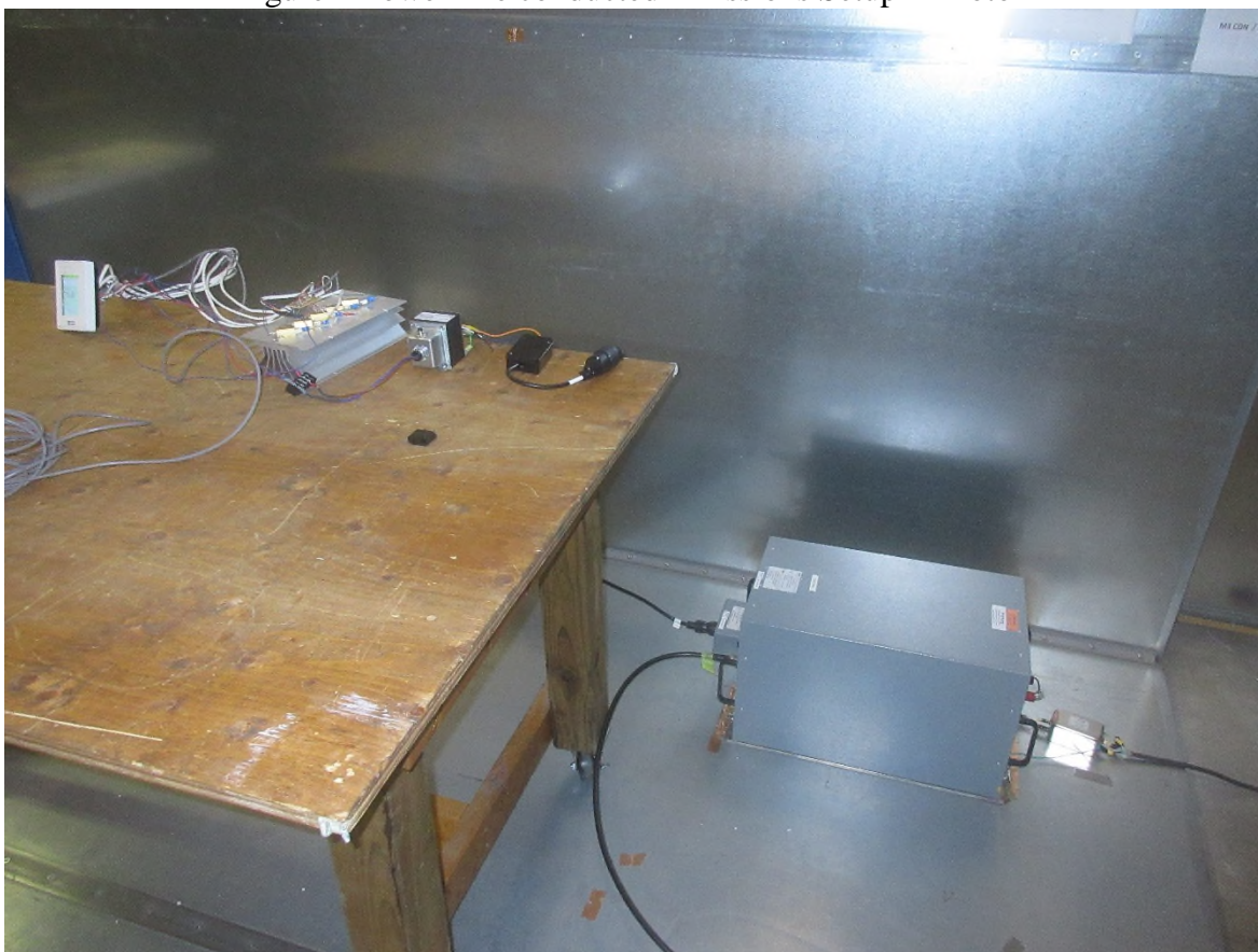
Figure 1 Power line conducted Emissions Setup – Photo 1
