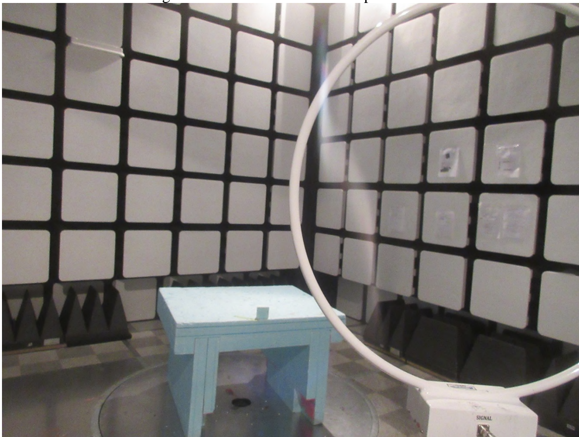
Figure 3 Radiated Emissions Setup – Photo 1
