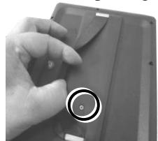
2. Slide the hand strap cover down in the direction indicated by the arrow.
