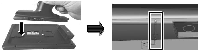
2. After ensuring the pistol grip is well attached to the tablet, push the pistol grip in the direction indicated by the arrow as shown in the figure.
