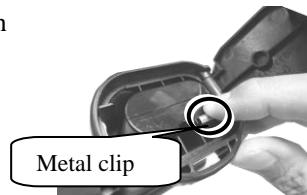
3. After having the rail on the battery pack aligned with battery clip, push down the battery pack into battery compartment.
