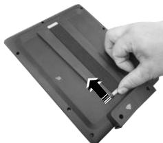
6. Fasten the hand strap cover onto the tablet using a screw.
