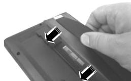
4. Make sure that the hand strap cover is well attached to the rear side of the tablet.
