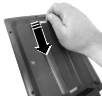
3. Remove the hand strap cover from the rear side of the tablet.
