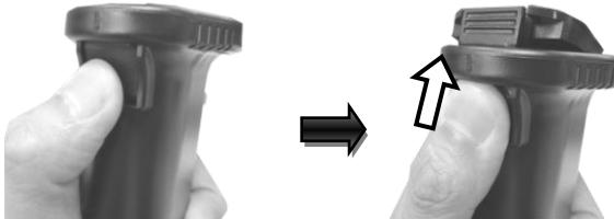
2. To replace the existing battery, gently push the metal clip outwards to release the battery. If you are installing the battery for the first time, please skip to the next step.
