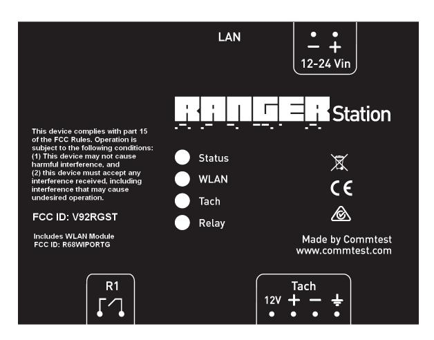
Label is printed on 8B35 0.25mm Polycarbonate backed by Scotch 467 Adhesive.
