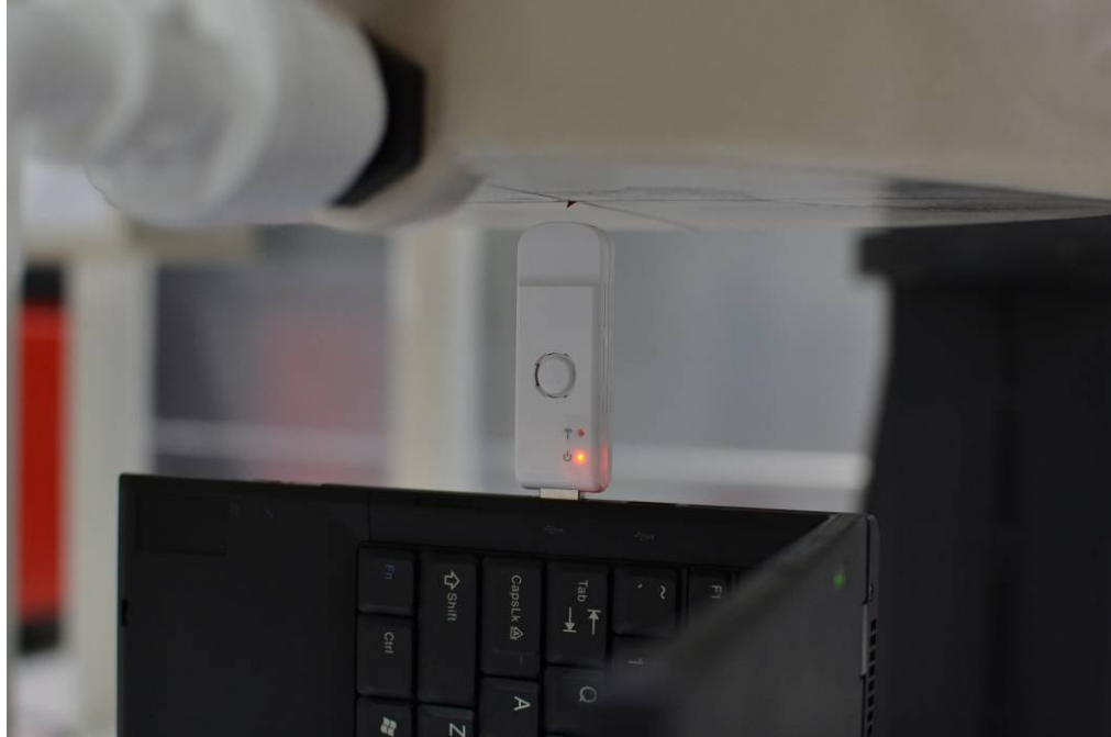
SAR Test Setup Photo 3 Tip at 0.5 cm
