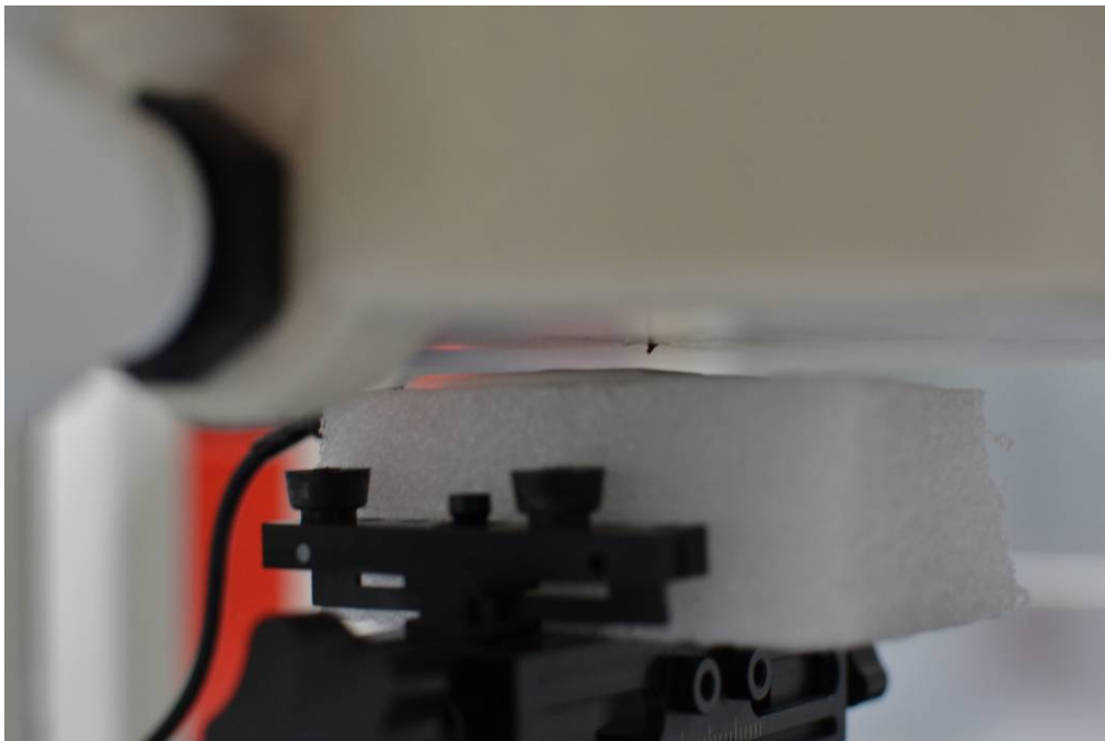
SAR Test Setup Photo 2 Horizontal Down at 0.5 cm
