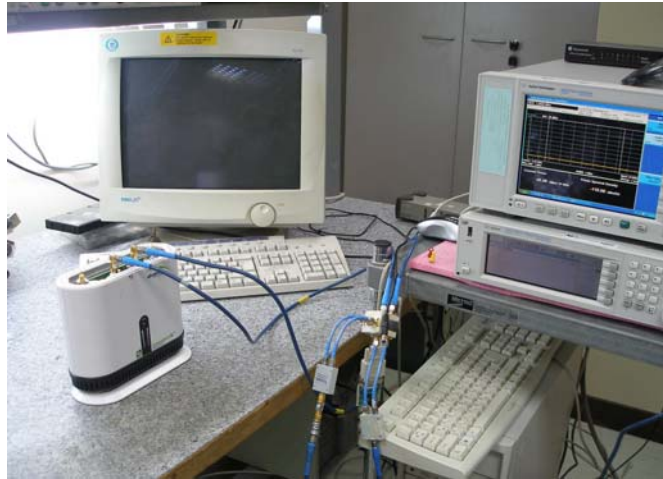
Photo 1. Conducted measurements. Test setup.
