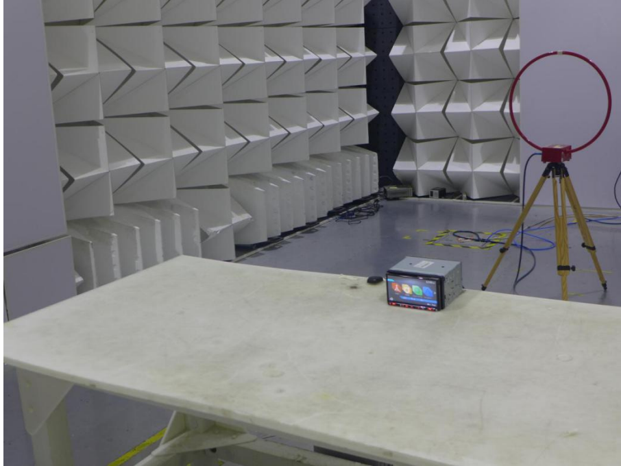
Radiated spurious emission Test Setup-1(Below 30MHz)
