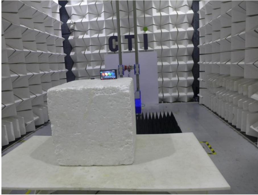
Radiated spurious emission Test Setup-3(Above 1GHz)
