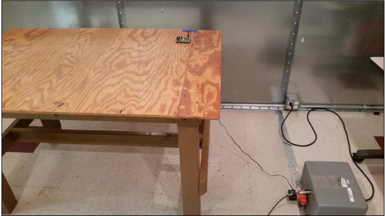
Photograph 2. Conducted Emissions, Test Setup
