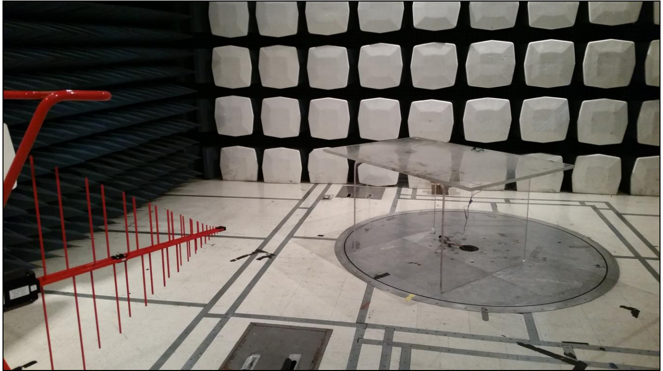
Photograph 3. Radiated Emissions, Test Setup
