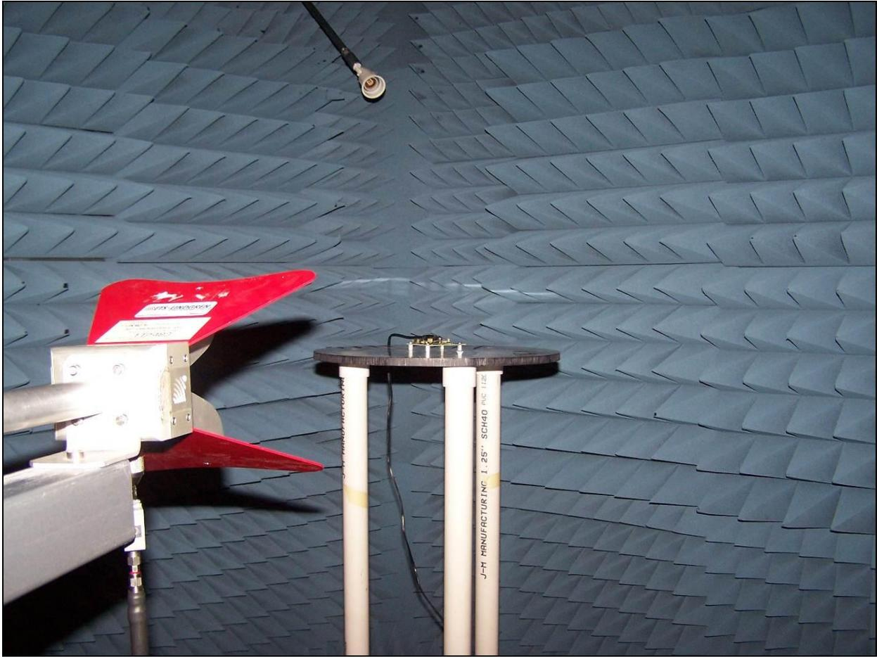
**Photograph 4. Radiated Spurious Emissions, Test Setup**
