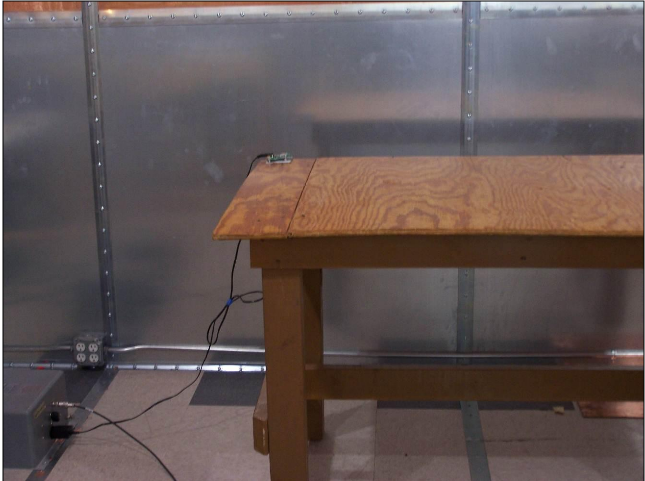
Photograph 4. Conducted Emissions, 15.207(a), Test Setup
