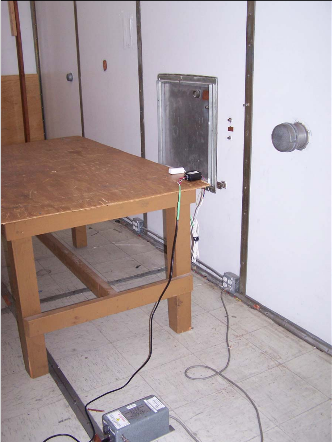
Photograph 2. Conducted Emissions Test Setup
