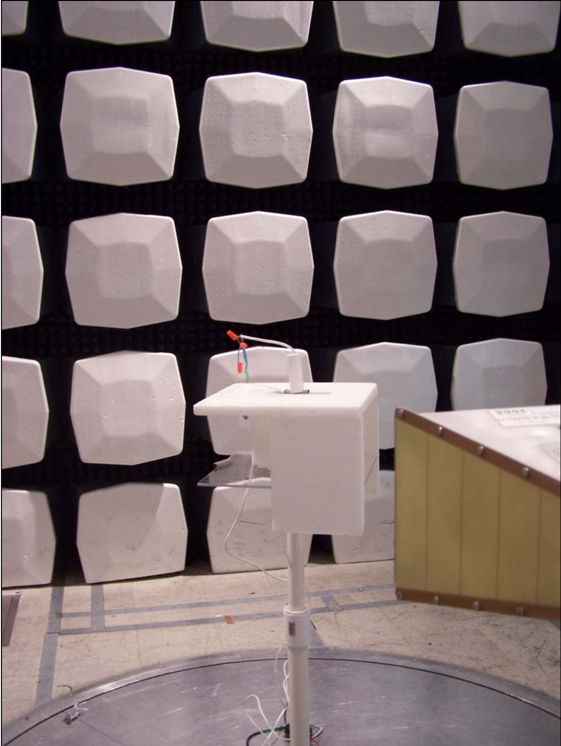
Photograph 1. Radiated Emissions Test Setup
