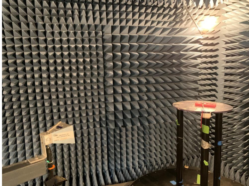
Figure 4: Radiated Spurious Emissions, 18 GHz – 25 GHz, Test Setup
