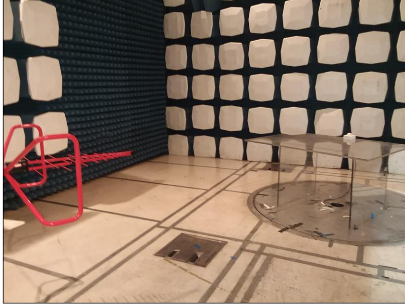
Photograph 2. Radiated Spurious Emissions, Test Setup, Below 1GHz
