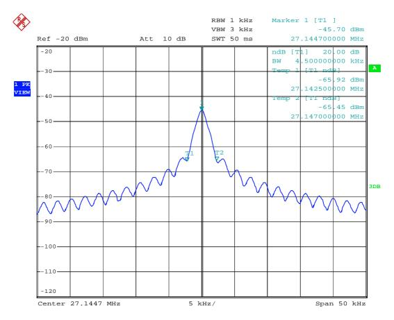
20dB Bandwidth: 4.5KHz (27.1425MHz to 27.1470MHz)
