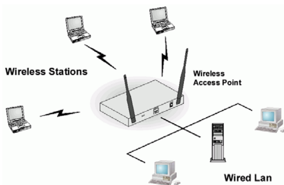
Figure 1: Wireless Access Point
