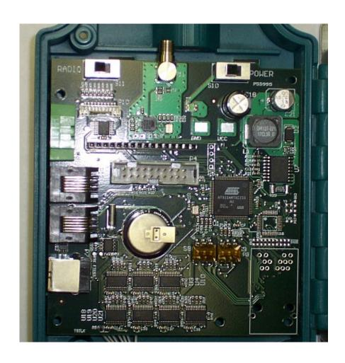
TPC IO device communication board w/ lcd front-
