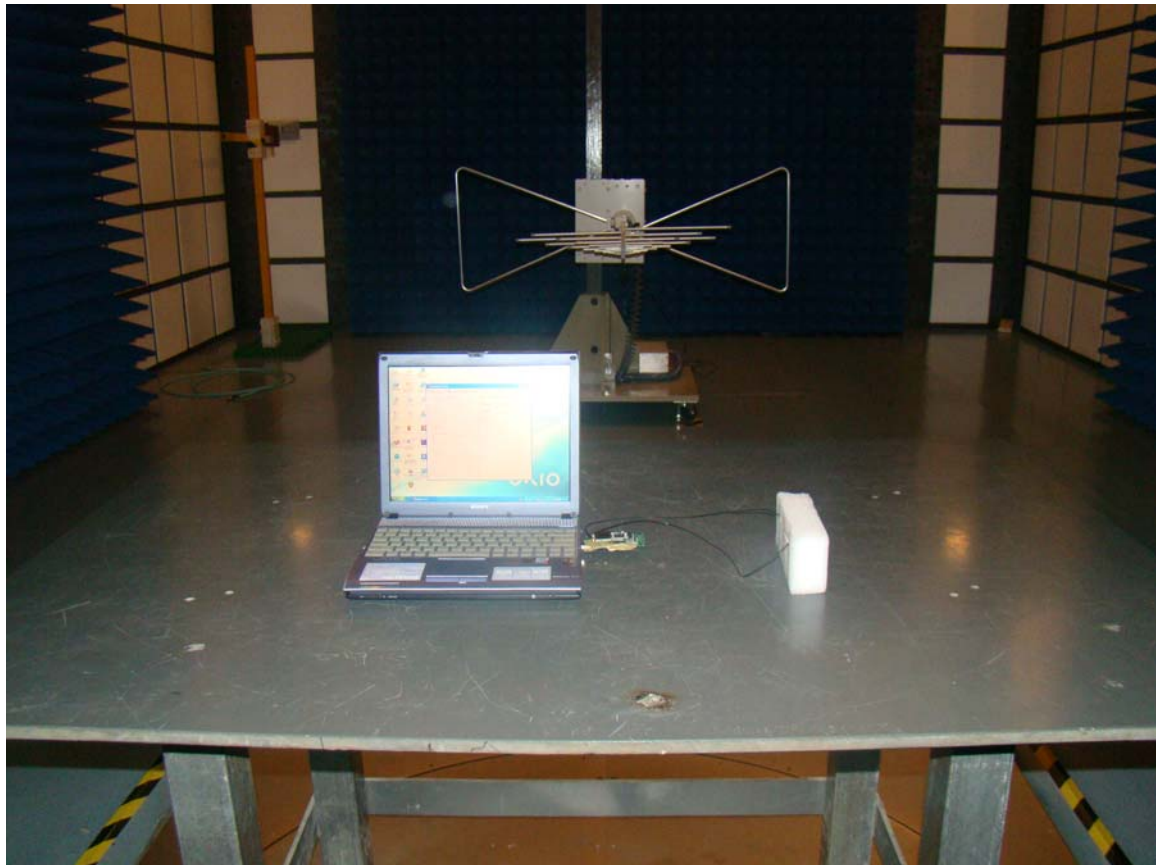
Radiated emissions test < 1GHz
