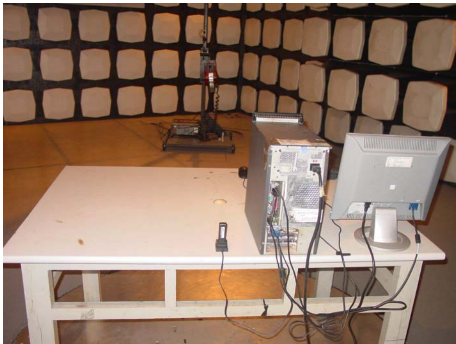
Figure 4 Test photo of Transmitter Spurious Emission (TX Mode 1000-18000MHz)
