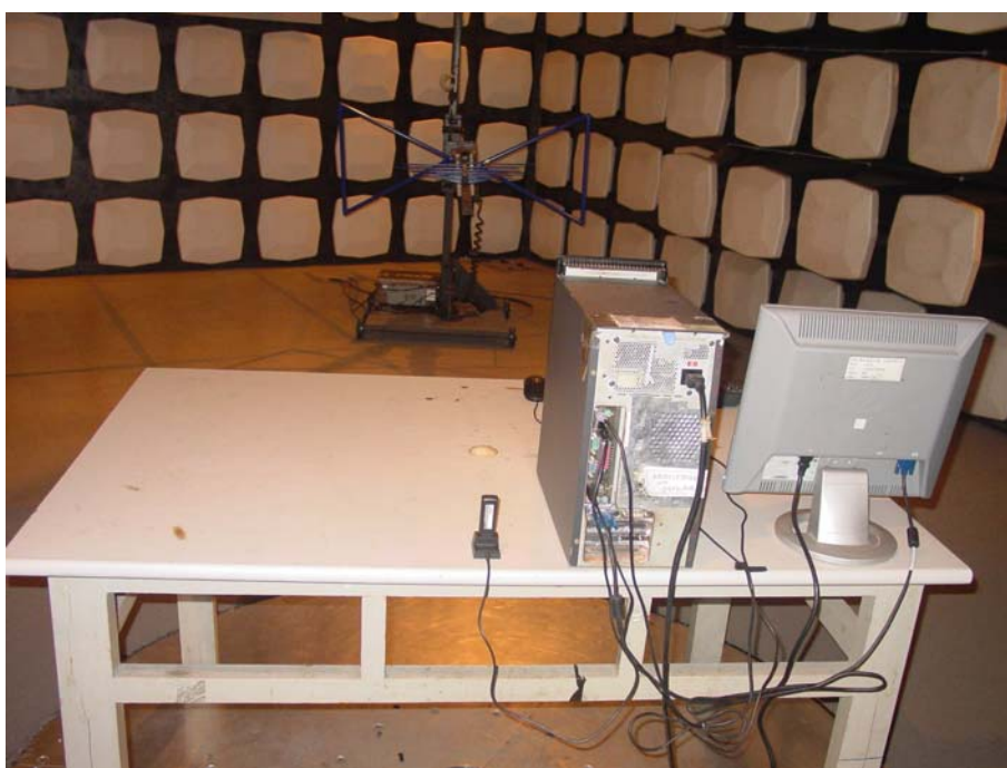
Figure 2 Test photo of Transmitter Spurious Emission (TX Mode 30-1000MHz)
