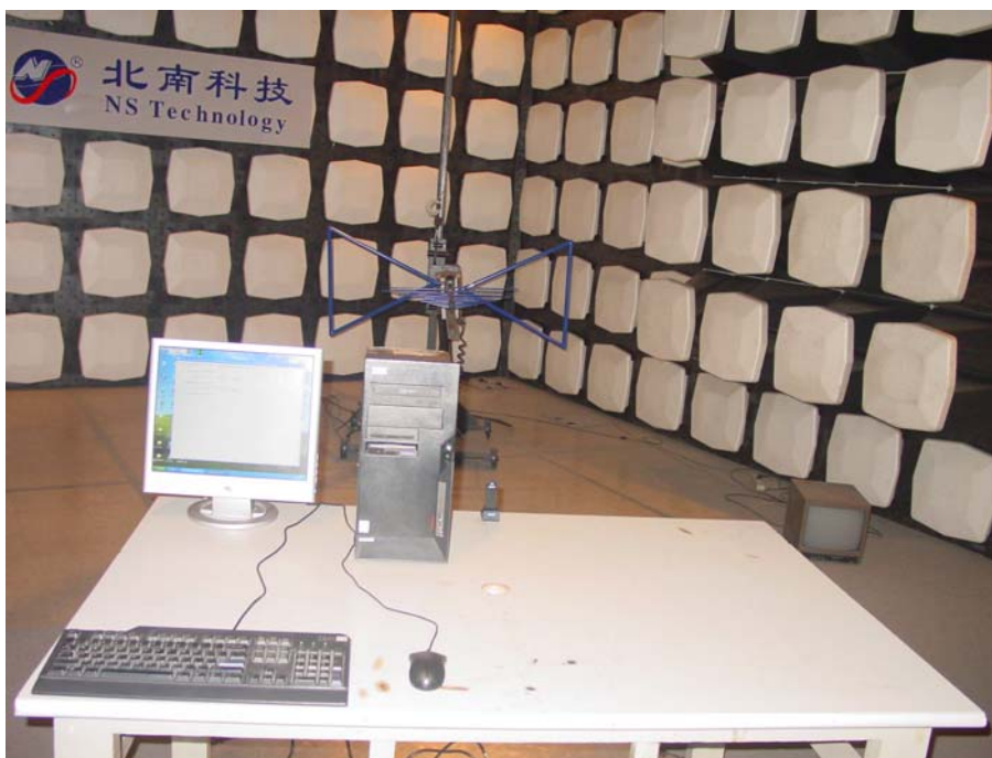
Figure 1 Test photo of Transmitter Spurious Emission (TX Mode 30-1000MHz)
