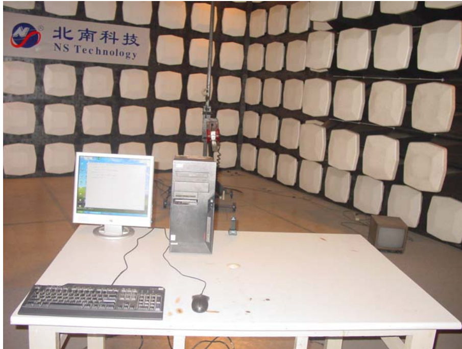
Figure 3 Test photo of Transmitter Spurious Emission (TX Mode 1000-18000MHz)
