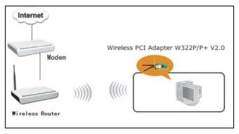
In this mode, W322P/P+ V2.0 serves as a client to receive the wireless signals to access the Internet.
