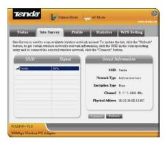
**Connect:** select one entry in the wireless network list and click the button to connect the device with the selected network.
