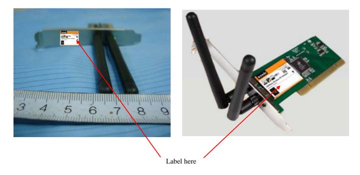
The label shown shall be permanently affixed at a conspicuous location on the device and be readily visible to the user at the time purchase (Labeling requirements per 2.925)
