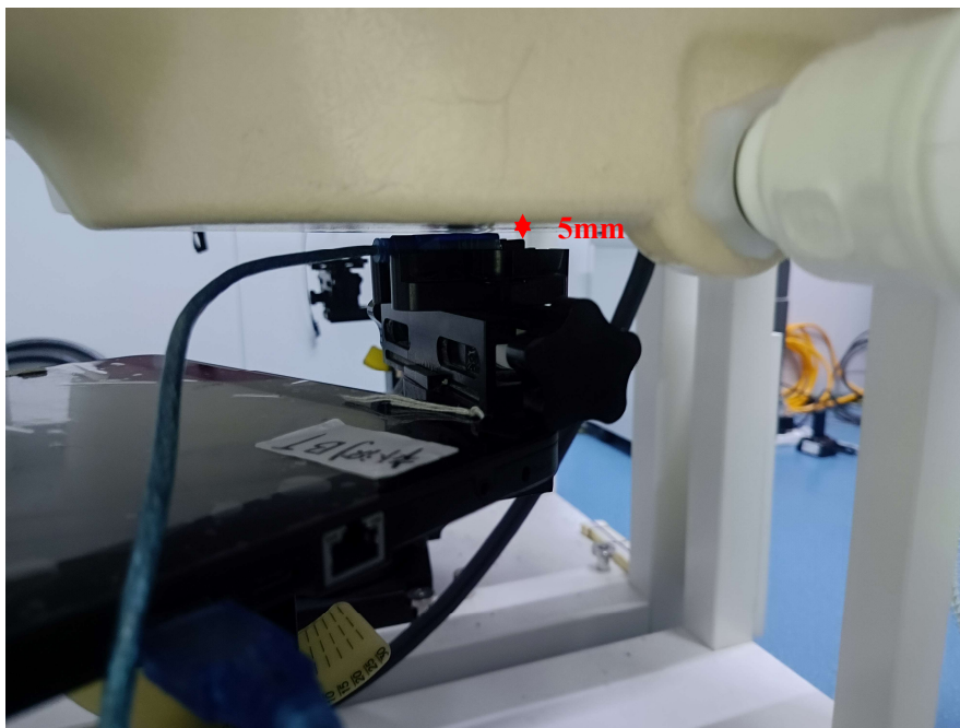
Horizontal-Down Adding USB extension cable Setup Photo (5mm)
