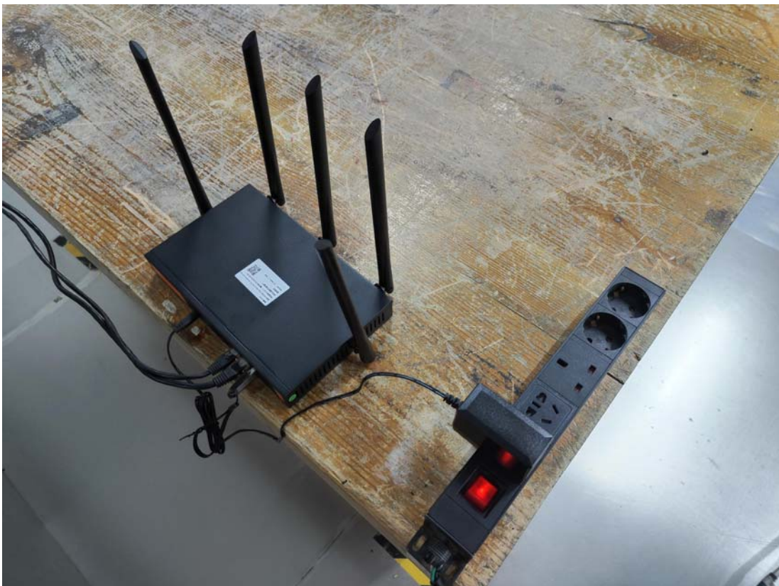
Conducted Emissions Side View
