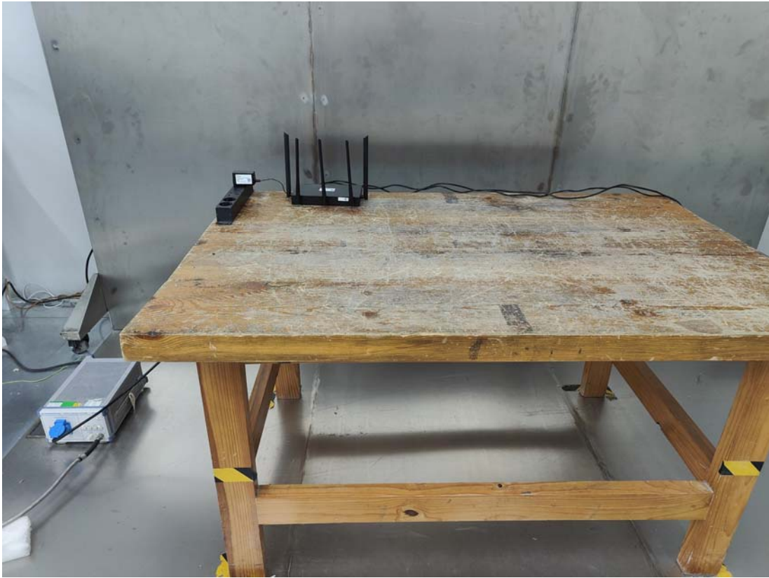
Conducted Emissions Side View
