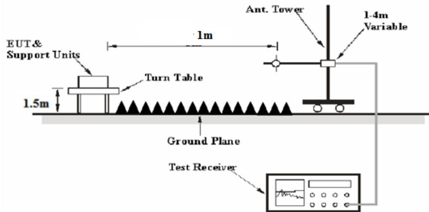
The radiated emission Below 1GHz tests were performed in the 10 meters chamber test site , above 1GHz tests were performed in the 3 meters chamber test site A, using the setup accordance with the ANSI C63.10-2013. The specification used was the FCC 15.209, and FCC 15.407 limits.
