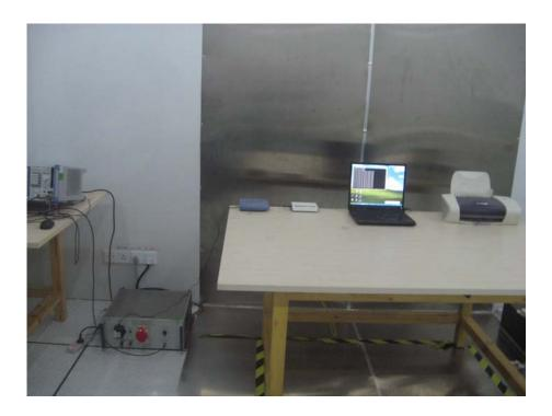
Radiation Emission Test Setup (30MHz to 1GHz)
