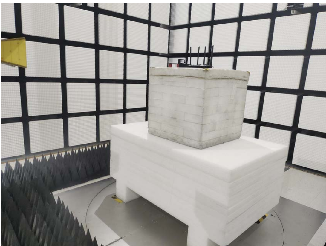
Radiated Emission Above 1GHz View
