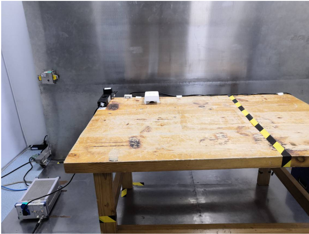
Conducted Emissions Side View-PoE Power Mode
