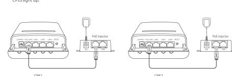
• Tips: • Automatic bridging only works for CPEs in factory settings. Peer-to-peer bridging takes effect within one minute after the CPEs start. Automatic bridging could fail if three or more powered CPEs in factory settings are placed nearby. When the CPEs are powered on using Ethernet cables, CATSe or better Ethernet cable is recommended and the length should not exceed 50 meters.
