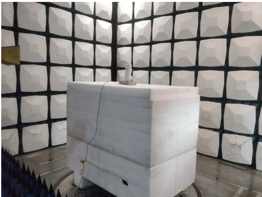
Radiated Emission Above 1GHz View
