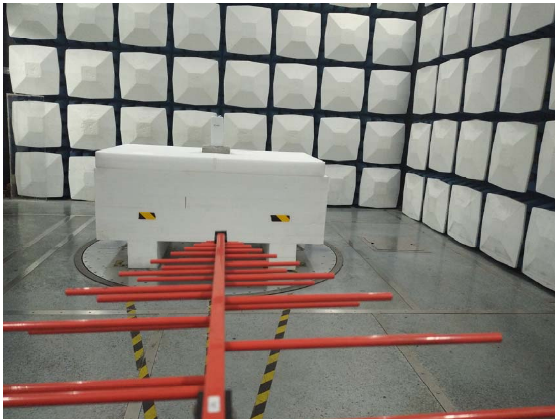
Radiated Emission Above 1GHz View
