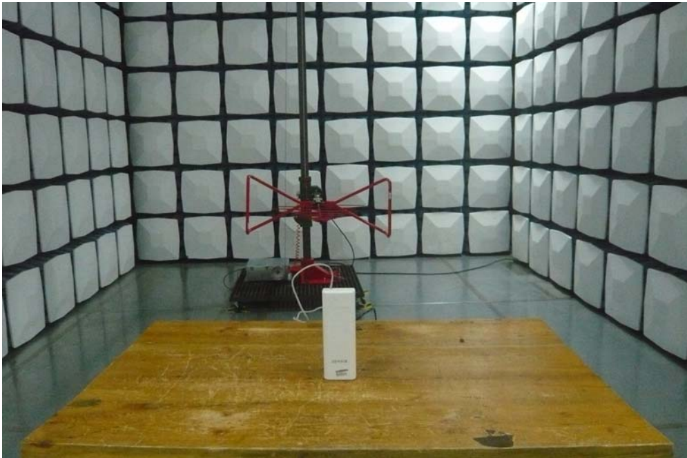
Radiated Emission View (Below 1GHz)
