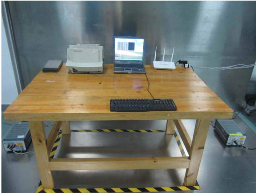
Conducted Emission - Side View
